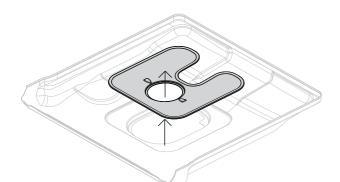
With the filter removed, carefully lift the filter plate up and out.
