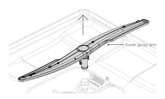
To remove the lower spray arm, lift it from the base of the dishwasher.
