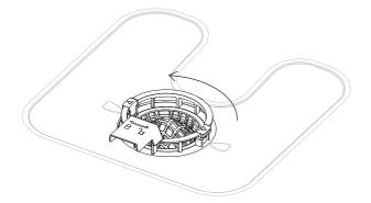
**1.** Twist the filter anti-clockwise to release. Lift to remove.
