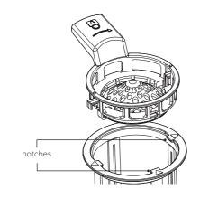
1. Align the filter cap with the notch on the filter base for one side. Press the button to settle the filter cap on the filter base for the other side.
