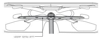
Do not remove the top spray arm for cleaning.
