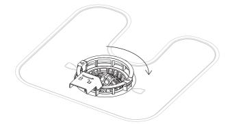
2. Place the drain filter back into the dishwasher base. Rotate clockwise to click into place.
