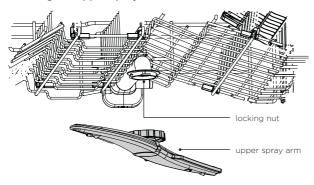
To remove the upper spray arm, turn the locking nut clockwise to release. Rinse the spray arm thoroughly under
