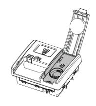
1. Lift the cover open and pour rinse aid into the opening. Do not fill past the MAX line. Take care not to spill any onto the door or detergent bucket.
