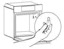
2. Once the bulb is replaced, ensure the glass cover is replaced. Ensure you disconnect the oven from the mains supply before you clean or change your light bulb.
