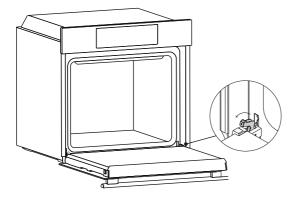
2. Rotate the hinge locks outwards. You may wish to use a screwdriver to grip the hinge.
