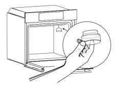
To remove your light bulb, undo the glass cover, unscrew the bulb and replace it with a new bulb of the same type.
