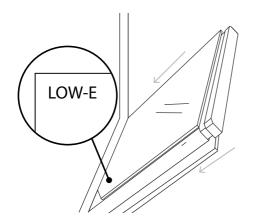
6. Once clean, carefully refit the glass and ensure the 'LOW-E' label is on the left side of the door, close to the hinge. The label will be inside the door.
