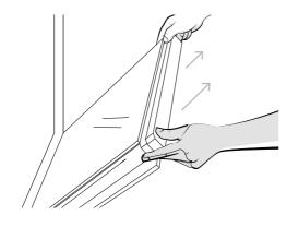
4. Remove the upper metal cover by pulling it upwards.
