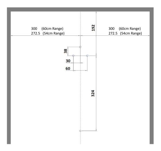
**Step 2**Fix the anti-tilt bracket with 3 screws and 3 anchors.
