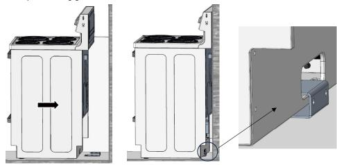
**Step 4**Remove drawer as defined in pictures. Pull out drawer by pushing the bar downwards on the right side and upwards on the left side.
