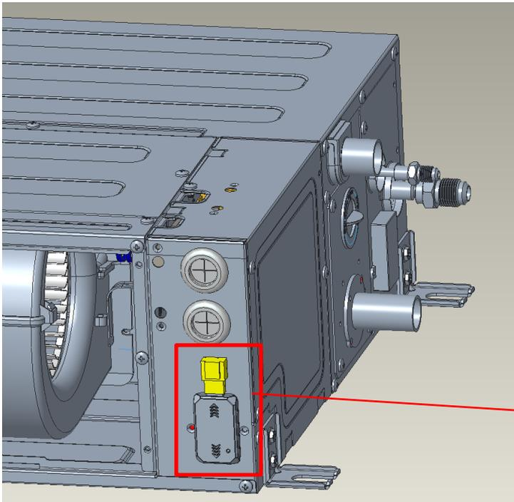
1. Install the Wi-Fi module into the place circled with red rectangle as shown in the picture. Use the 3M double side tape to fix the Wi-Fi module.
